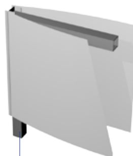
Aluminium or steel profile 60 x 60 x 4mm Aluminium oder stahl profil 60 x 60 x 4mm
