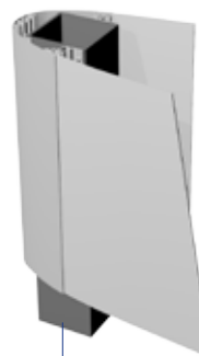
Aluminium or steel profile 80 x 80 x 4mm Aluminium oder stahl profil 80 x 80 x 4mm
